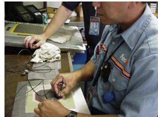
NDI using pitch-catch ultrasonic technique
