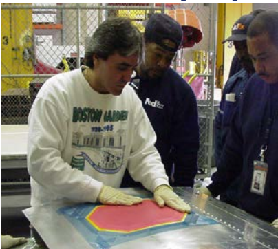
Applying doubler to cleaned surface
